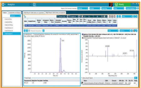
TOF MS and Information Dependent TOF MS/MS acquisition delivers reliable unknown identification of drugs in forensic samples.
