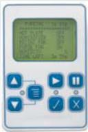
The electronic control system includes easy on-screen functions to programme the Purge Cycle, Manual Contact Override, Contact Time and RH Sensor settings which are easily calibrated and also allow different values to be set.
